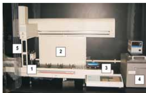
Figure 2. The Beckman Coulter BioMek® 2000 Laboratory Automation Workstation with modifications for DNA extraction using the DNA IQ™ Extraction System by Promega including: 1) Left Module (contains Tool Rack for holding MP200 pipetting tool- 8-channel, P200L pipetting tool-single channel, Gripper Tool, and other optional pipetting tools), 2) Base Module, 3) Right Module (contains shaking platform), 4) Circulating Water Bath (for heating Thermal Exchange Unit), and 5) Disposal Area.
