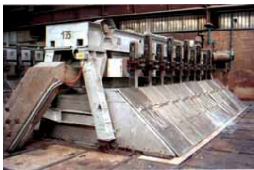
Figure 2. Modernized electrolytic cells and new way of alumina dosage.
